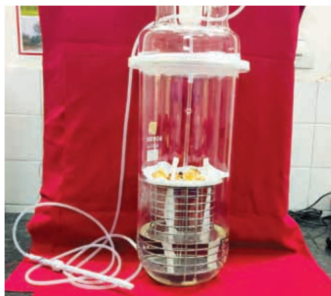
Assembly of culture vessel to develop a prototype of bio-reactor containing medium and callus culture
