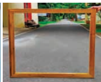
Bamboo lumber (using bamboo strips and crushed bamboo) made from different bamboo species
