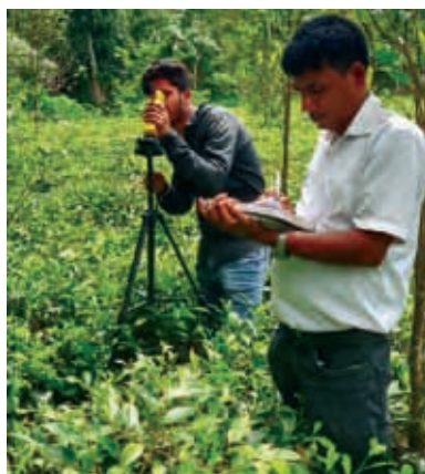
Measurements of trees with the help of electronic BAF Scope
