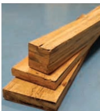
Bamboo lumber (using bamboo strips and crushed bamboo) made from different bamboo species
