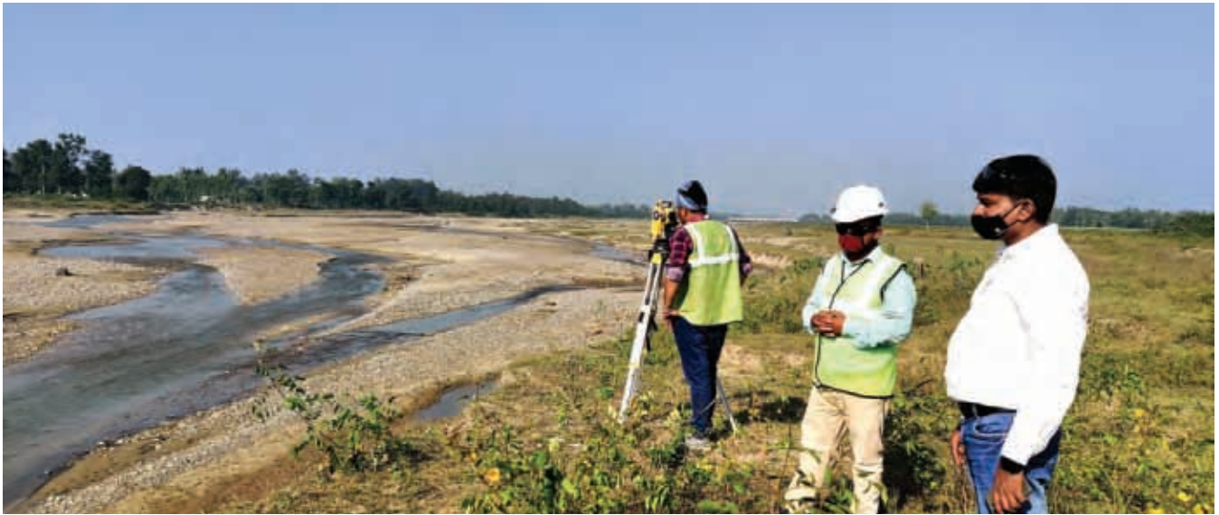
Topographical survey of the study area using Total Station
