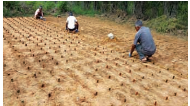
Control, CCB and Six neem formulations treated samples installed in field experiment at Nallal, Karnataka
