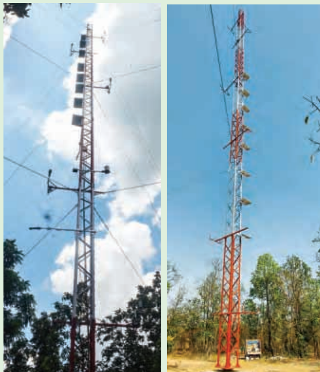
Carbon Flux Towers installed in Madhya Pradesh and Chhattisgarh
