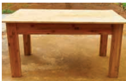
Bamboo lumber (using bamboo strips and crushed bamboo) made from different bamboo species
