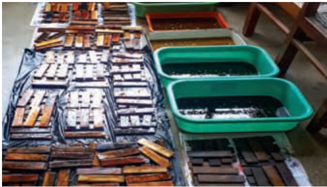
Control, CCB and Six neem formulations treated samples installed in field experiment at Nallal, Karnataka
