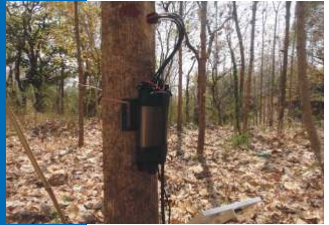
Sap flow meter installation on Tectona grandis tree
