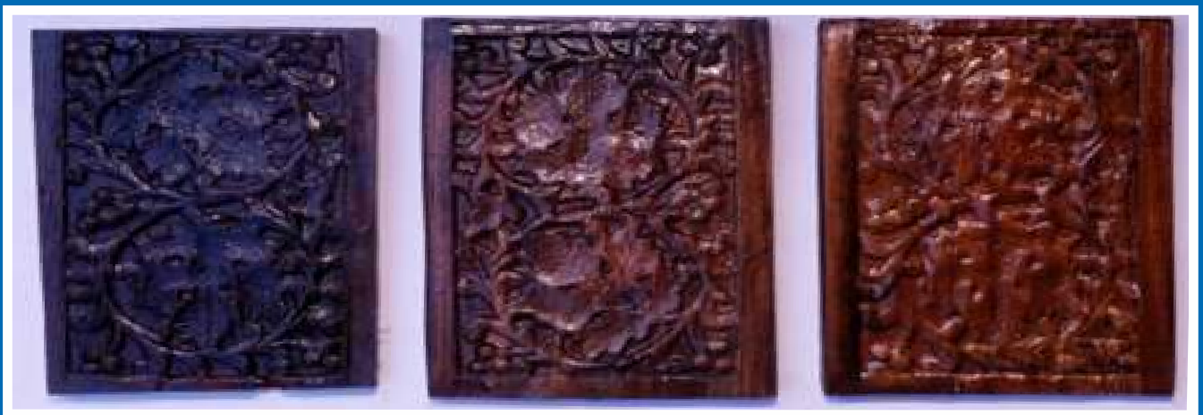
'Die-tool' imprinted wood blocks using THM treatment
