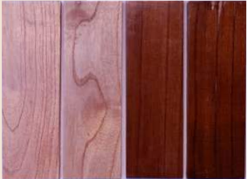
Raw wood of M. dubia and it is modified using Thermo-Hygro-Mechanical process
