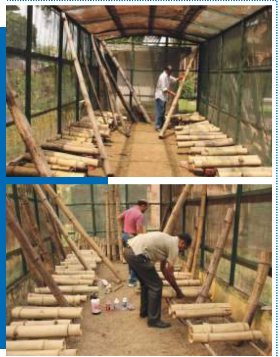
Preservative treatment in dry bamboo
