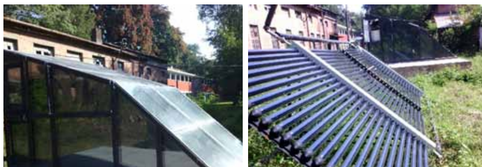
Modified solar kiln with phase change material as solar storage system
