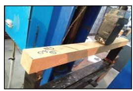
**Figure 14.a**) Preparation of samples from wood logs, and b) Testing of mechanical properties.
