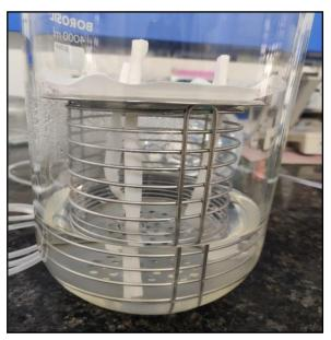
**Figure 15.** Assembly of culture vessel to develop a prototype of bio-reactor containing medium and callus culture.
