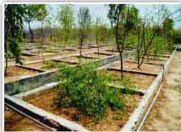
Lysimeter experiment for phytoremediation
