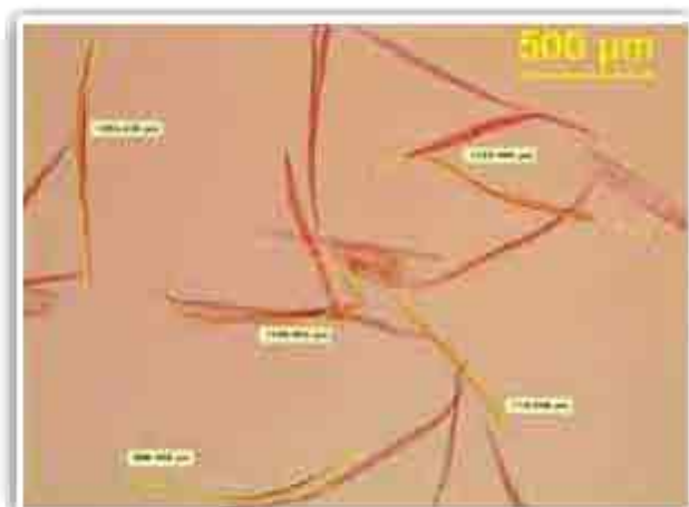
Measurement of wood fibre length in 5X magnification using Leica microsystem EC 3 (A) Wood fibres in unmeasured form (B) Measured wood fibres
