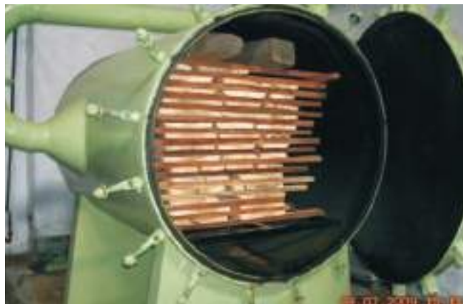
Vacuum Kiln for Timber Drying Developed by FRI, Dehradun
