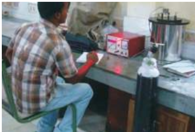
Calorific Value Estimation Using Bomb Calorimeter
