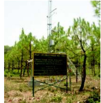
Micrometrological Station in F.R.I. Campus
