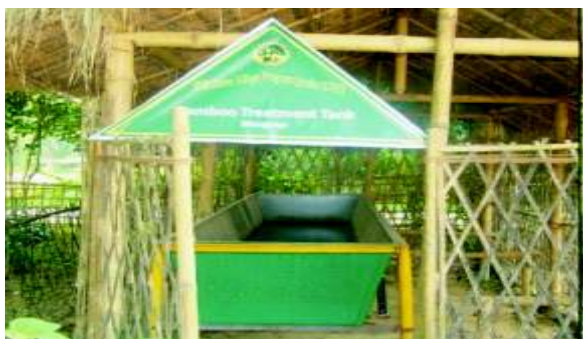
A Bamboo Treatment Tank
