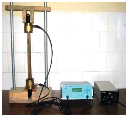
Ultrasonic Wood Tester to detect defects in wood
