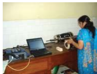
FFT analyzer to record sound waves from Dholak
