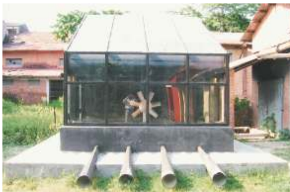
Modified Solar Kiln
