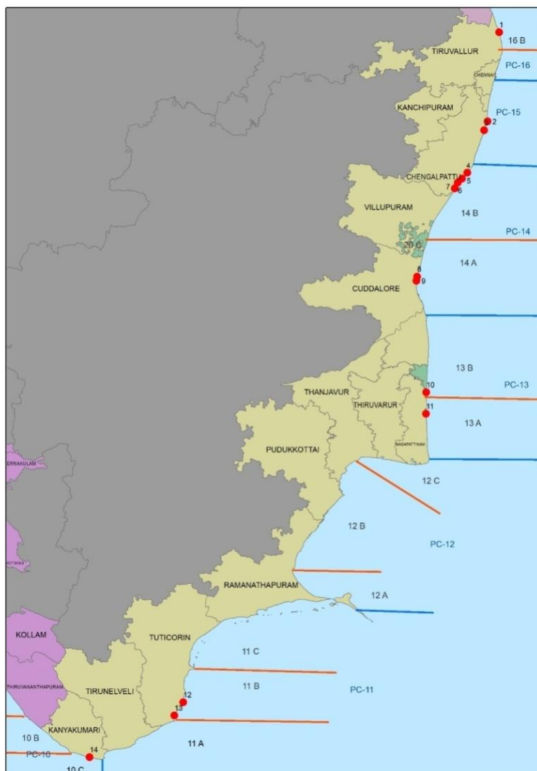
Figure 3. Erosion hotspots along the coast of Tamil Nadu based on the shoreline Change analysis and numerical simulations
