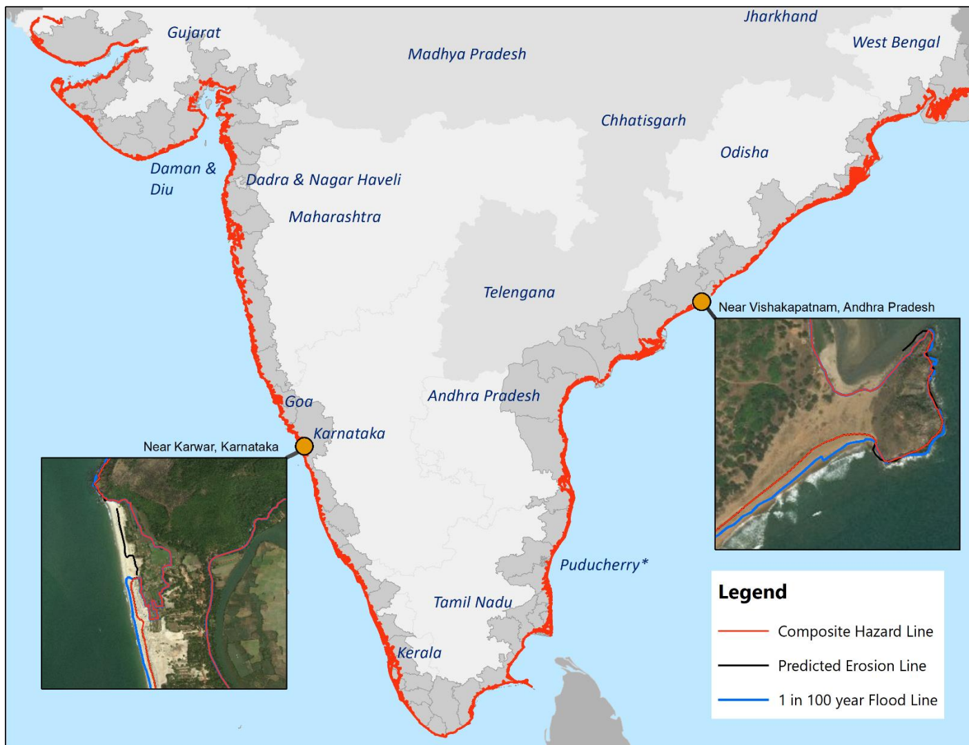
Figure 6: Composite Hazard Line for the Coast of India. Insert: West coast: Near Karwar, Karnataka and East Coast: Near Visakhapatnam, Andhra Pradesh showing 1 in 100-year flood line, 100-year predicted erosion line and composite hazard line
