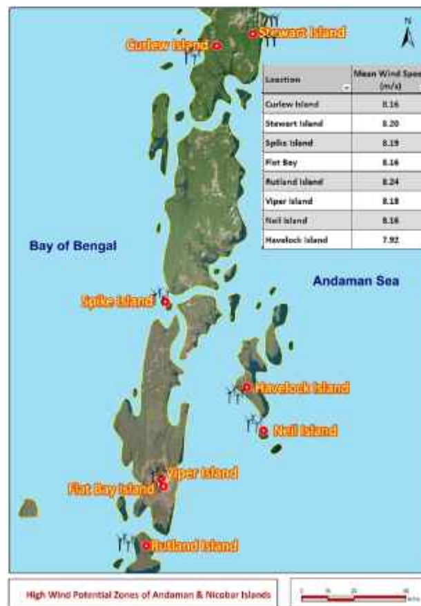
Fig. 4. Islands with high onshore and offshore wind power potential in Andaman & Nicobar Islands
