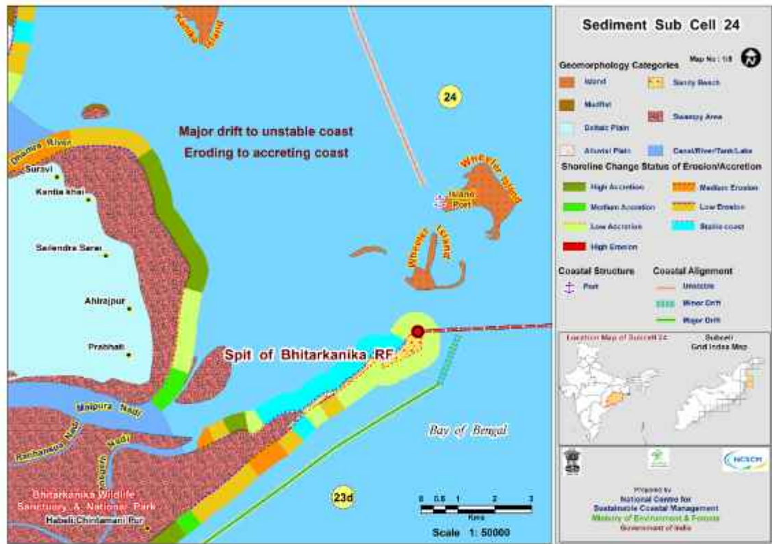
Fig. 14. Delineation of sub-cell on the basis of littoral drift
