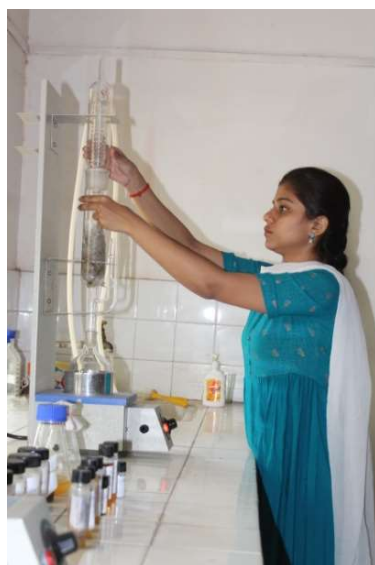
Fig. 40: Extraction of seed oil using Soxhlet Apparatus.
