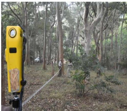
Fig.2. Measurement of tree diameter at different height segments of Terminalia arjuna at Balod forest division, CG using Basal Area Finder (BAF) Scope.
