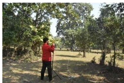
Fig.8 Measurement of tree diameter at different height segment at Bastar forest division using Basal Area Finder (BAF) Scope
