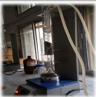
Fig.40 Extraction of crude extracts using Soxhlet Apparatus
